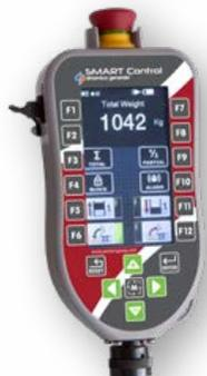
The **Smart Control** can be placed in the tractor or loader for reading the weights, reading level of unloading doors or conveyor height and/or for control of all hydraulic functions. You can also combine functions such as starting the conveyor and opening the unloading door with one simple push on the button. Also the activation of a **Power Booster** is a possibility.
